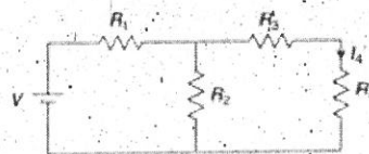
When voltage source V is acting alone
