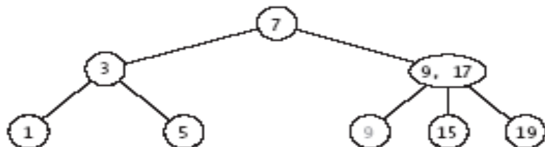
FIGURE 11.44 Removing 11 from the 2-3 Tree (Step 1)
